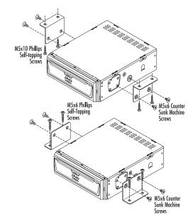
Figure 12. Horizontal mounting of VS715.
